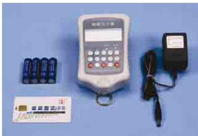
Figure 43 The IC card and card writer
